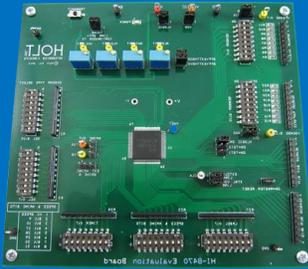
ADK-8475/6 → ARINC 429 Receiver with parallel and serial outputs Evaluation Board
